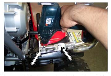
Bit. After Drilling Holes, Secure the Flat Plates to the Foot Pegs using the 6mm Flange Bolts, 6mm Flat Washers & 6mm Nylock Nuts supplied.
